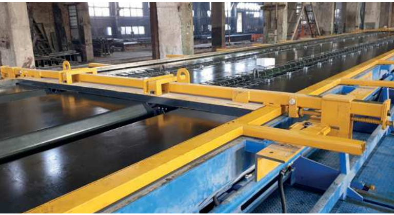
TT mould ready for casting
