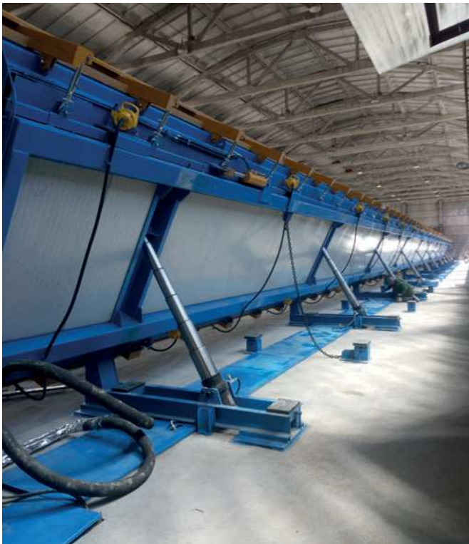
Back View of tilting table with vibration plant and hydraulic displacement of upper side detail
