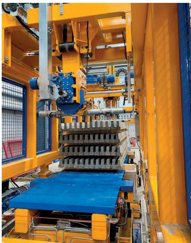
Rotator stacker in operation
