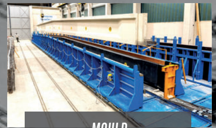
MOULD for Prestressed Beams
