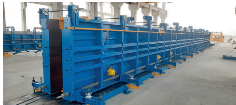
Mould sides for I beams
