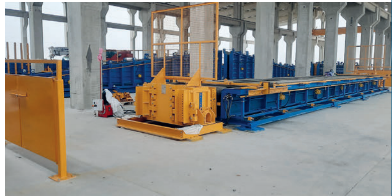
Self-reacting mould for TT slabs
