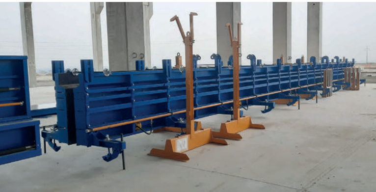
Mould sides for T-beams
