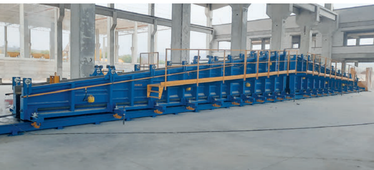
Mould sides for double slope beams
