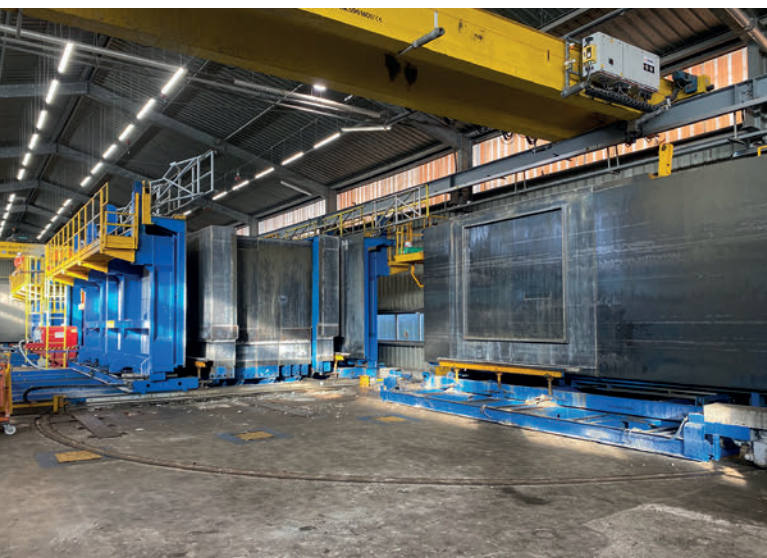
Production of free-standing 3-dimensional modules with PPVC technology
