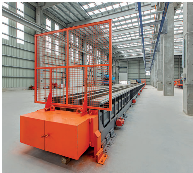
Mould for purlin beams
