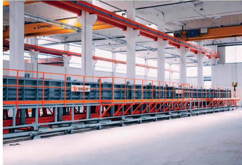
Multisection column formwork
