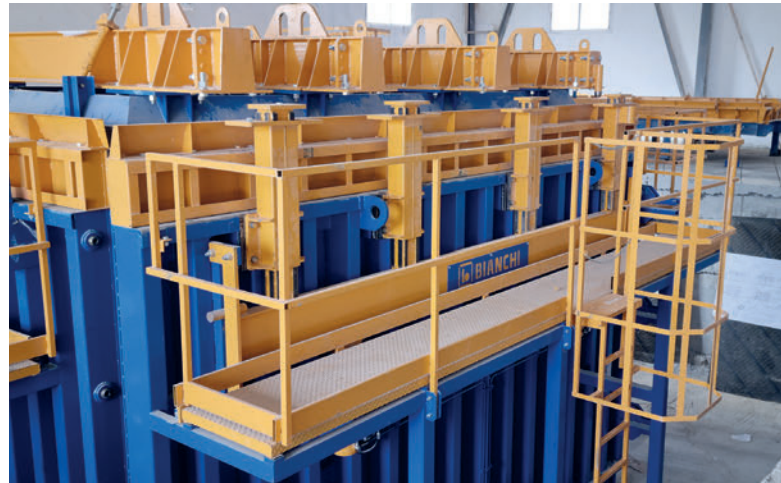
Mould with walkways and handrails
