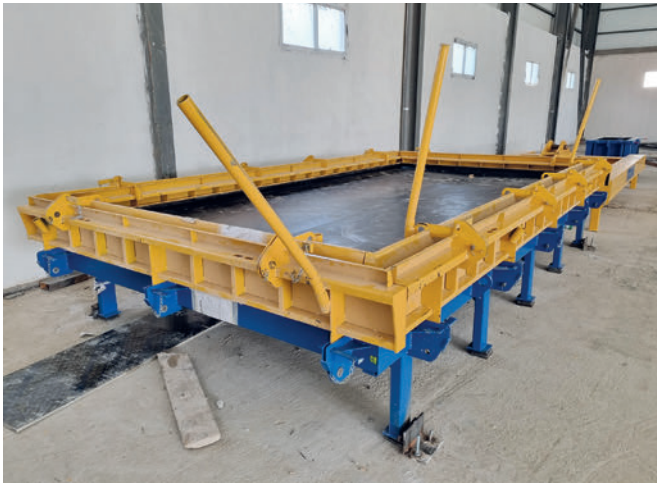
Fixed table to produce the roof element
