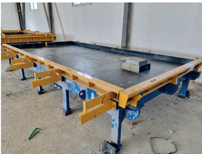
Fixed table to produce floor slab
